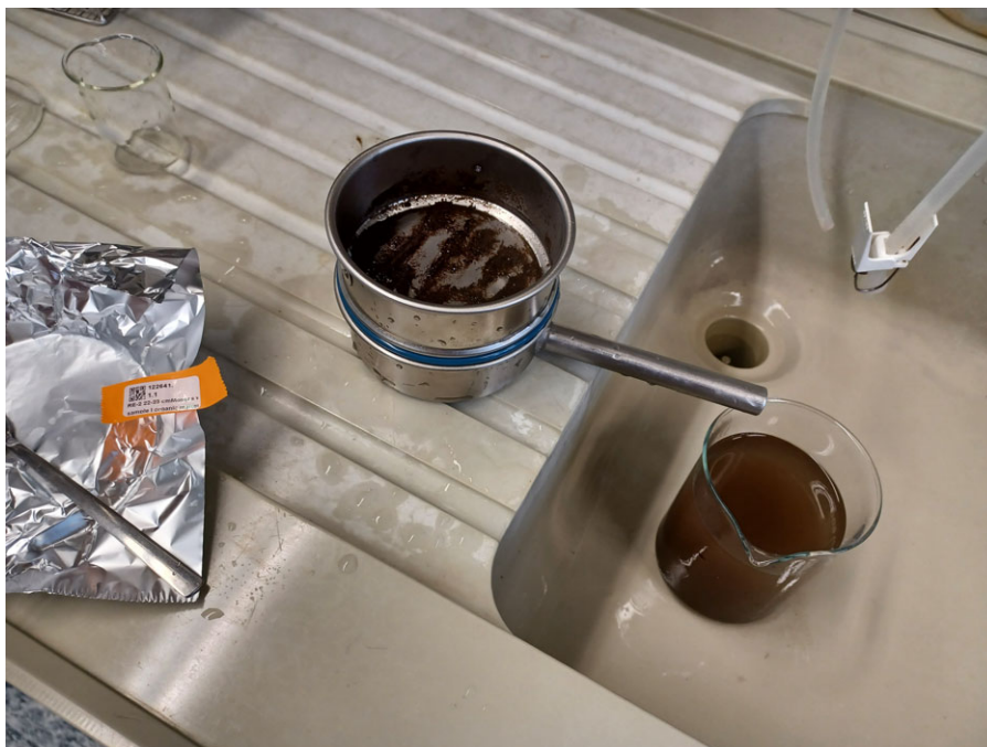
Figure 1 Setup for wet sieving of sediment and peat samples. The fine fraction ( <125\ \mu\text{m} or 150\ \mu\text{m} ) is collected in a glass beaker. The larger fraction (top sieve) can be investigated under binoculars.
