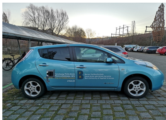
Figure 1: Research e-vehicle Nissan Leaf of the PV LAB at BFH (Burgdorf-Switzerland) showing photovoltaic reference cell measures irradiance levels on the right side of the car. Source: PV LAB at BFH.
