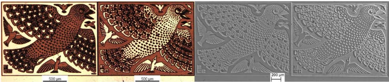
Figure 10: Comparison of the microscope image with the SEM image, 120 mW, 300 kHz, 3 µm pitch, 30 layers 14
