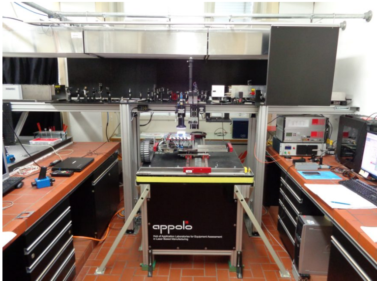
Figure 8 Lab scribing machine with optical experimentation platform installed at BUAS application lab.
