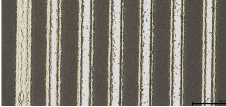
Figure 15 Robustness of the high-throughput P2 process with respect to changes of the focal position. Between scribing of each of the lines the focal position was shifted by 1 mm. All but the leftmost scribe show successful removal of the CIGS without Mo damage and thus valid P2 scribes.
