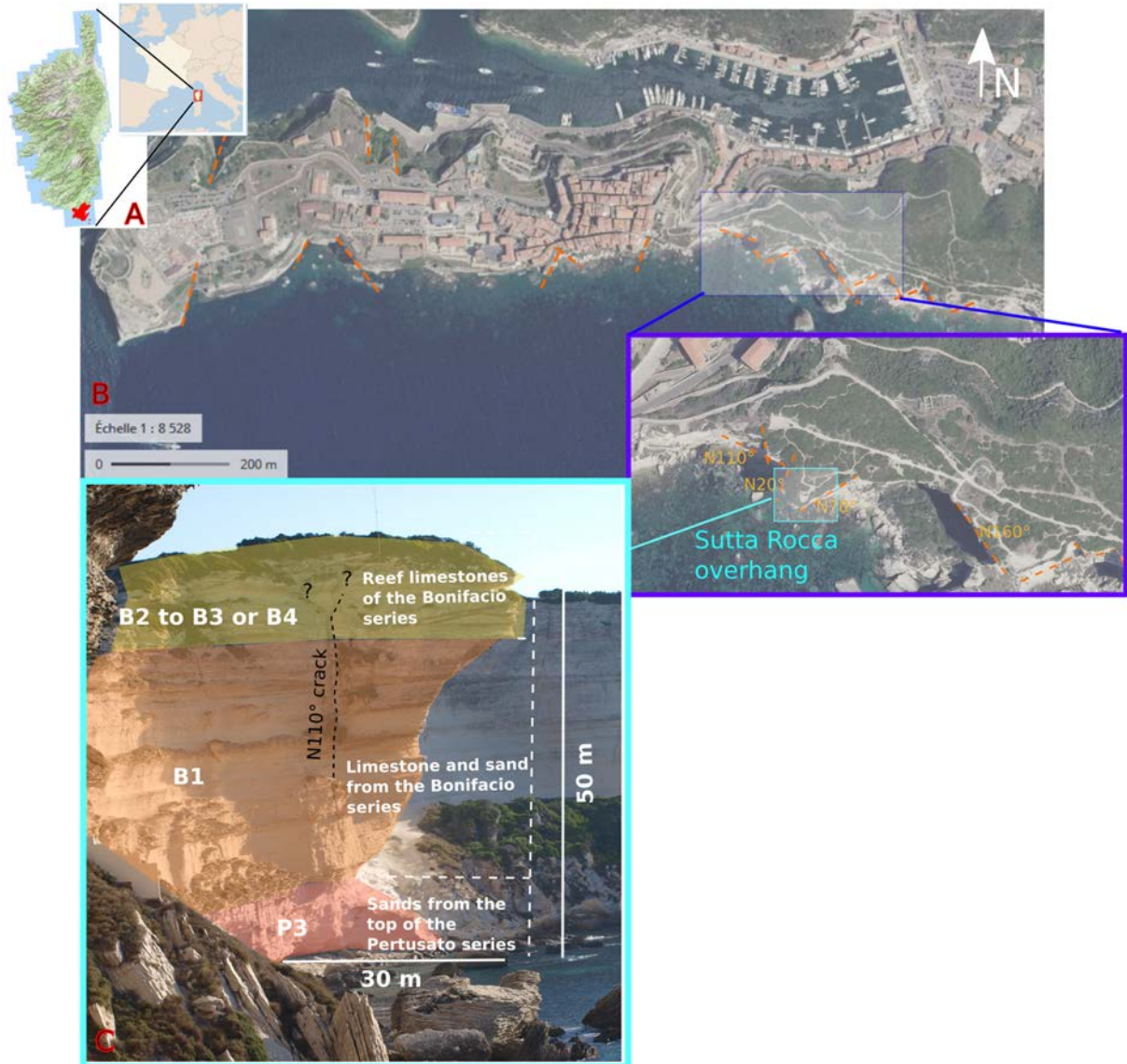
Figure 1. (a) Location map of the study area at the southern tip of Corsica island in the Mediterranean sea. (b) Detailed aerial view with the mapped faults of the Bonifacio formation (orange dashed lines). The coastal morphology is the result of erosion combined with tectonic accidents. Zoom-on the area of the Sutta-Rocca overhang. (Aerial photo Géoportail.) (c) Sedimentary sequence of the Sutta-Rocca overhang interpreted after Reynaud et al. (2013). From bottom to the top, unit P3: sands from the top of Pertusato series, unit B1: calcareous and sandy layers of the Bonifacio series and units B2–B4: reefal calcareous rocks of Bonifacio series. The vertical N110° crack is marked by the dashed black line. The colour version of this figure is only available in the electronic edition.
