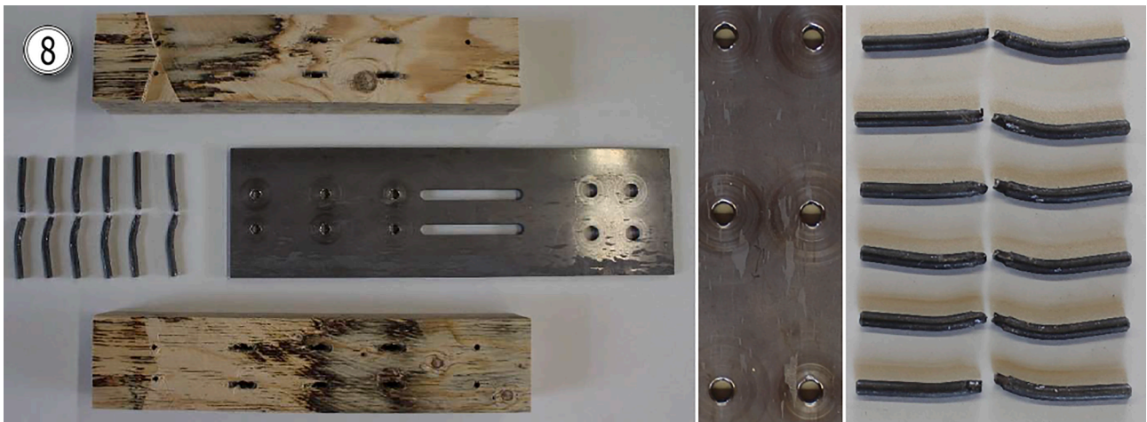
Fig. 18. Individual parts of the specimen 2S-6d8-R-c.3 after the cyclic test.
