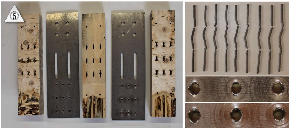
Fig. 14. Specimen 4S-9d6-RK-c.2 – Left: Timber members and steel plates - Right on the top: Dowels (failure mode 3) – Right on the bottom: Holes with crushed rounded edges. (The symbol left on the top means that both notch effect restraining measures have been taken).
