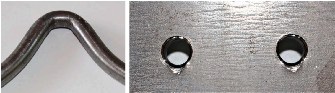
Fig. 16. Plastically deformed dowel, rounded and crushed plate hole edges after the monotonic test, both pictures from the specimen 2S-6d8-RK-m.1b (see Fig. 15 Force-displacement diagrams of both connections of the specimen 2S-6d8-RK-m.1).
