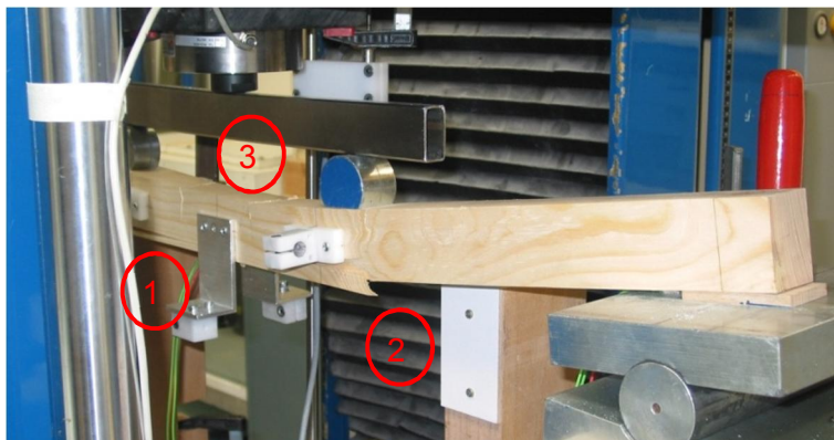
Figure 73: Specimen 14 shortly before complete failure (the force strain graph is presented in Figure 72) 1: first partial failure, 2: second partial failure, 3: strong crushing
