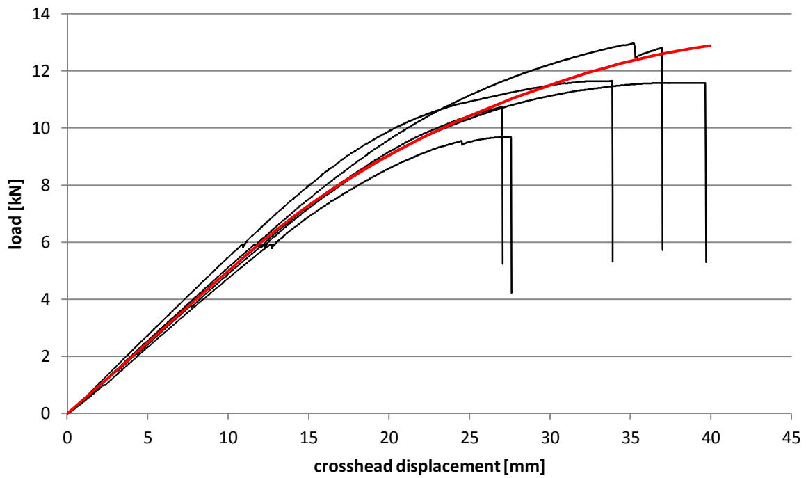
Figure A 4: Load as a function of the crosshead displacement of Sample C ( black: experimental measurements; red: FEM)
