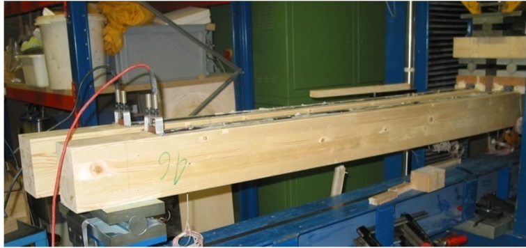
Figure 75: Cambering of two beams in Series 2 with the cables of the carboheater clearly visible on the left
