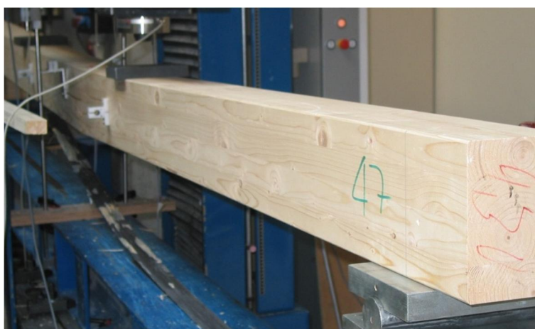
Figure 93: Specimen 47 after complete failure and unloading. The delamination of the CFRP-lamella was possibly the result of a partial failure.
