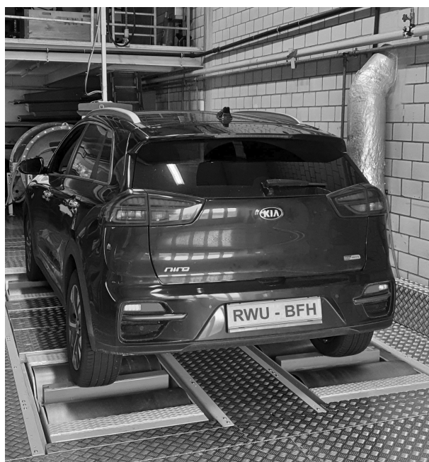
Figure 2. Kia e-Niro on the chassis dynamometer at Berner university of applied sciences.
