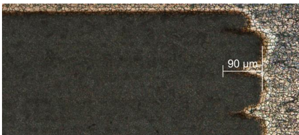
Fig. 17: Right border of the machined rectangles with periodic structures of dimension 90\ \mu\text{m} and a period of about 100\ \mu\text{m} .
