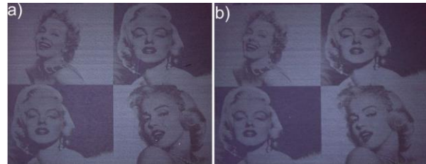
Fig. 14: 2 \times 2 marked picture on the a) left side and b) right side of the 17 \text{ cm} long marked area. The length of a single picture amounts 10.6 \text{ mm} .
