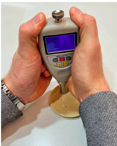
Fig. 5. Shore D hardness measurement performed on an adhesive sample.
