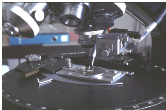
Fig. 3: Photograph showing the diamond micro-drill mounted on a conventional optical petrographic microscope.
