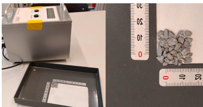
Fig. 5. Scanning coarse aggregate texture with Ames Engineering 9400HD 3D laser scanner.
