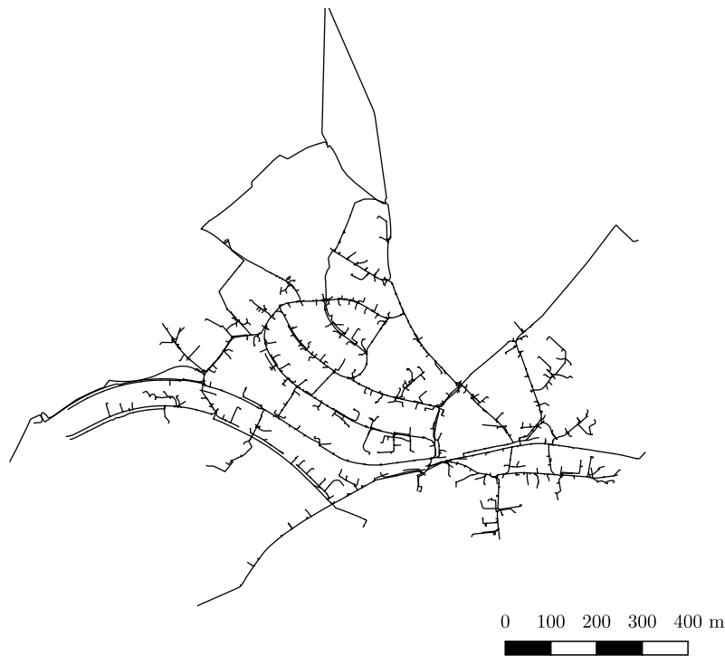
Figure 7.2.: Overview of the electricity network
