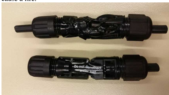
Figure 9: Failed Cross interoperability PV connectors Lumberg-MC of a BIPV-installation
