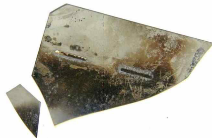
Figure 12: Silicon particle in the farmland – no further restriction for the use of the farmland
