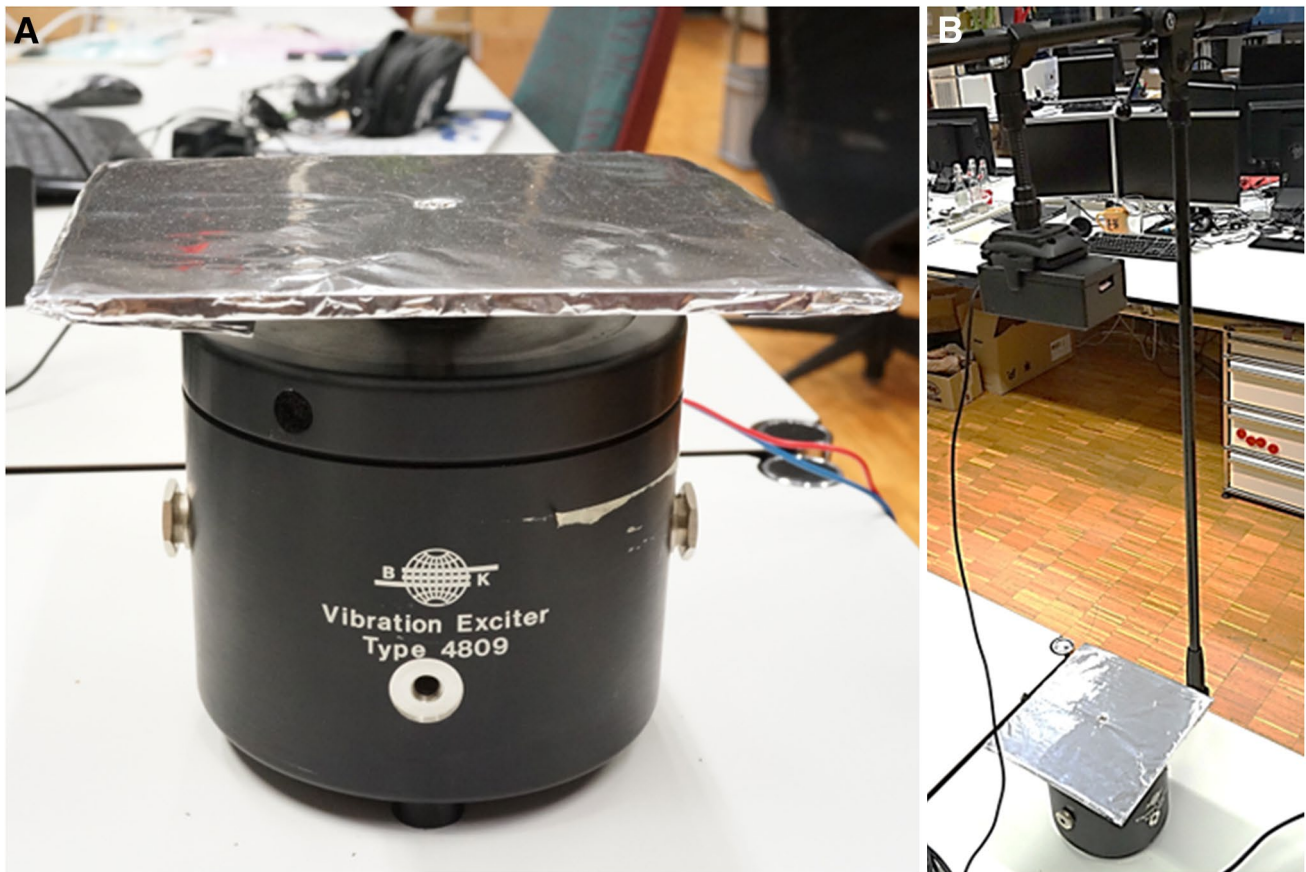
Fig. 4 Test bench setup: exciter with the vibrating surface mounted on top (a) and the prototype positioned (b)
