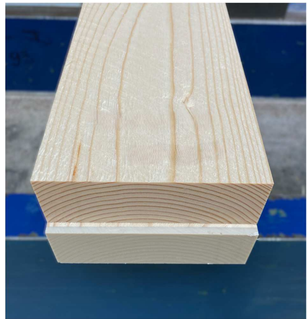
Figure 6. Representative adhesive failure mode.
