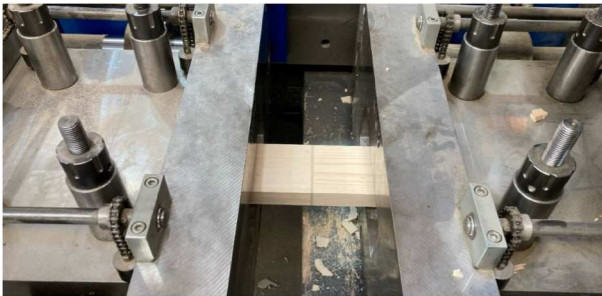
Figure 5. Test specimen in the tensile testing machine.
