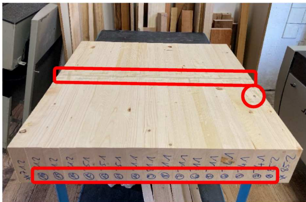
Figure 2. End-grain bonded glulam element: circle = injection hole; upper rectangle = casting resin joint; lower rectangle = numbering of the lamellae.
