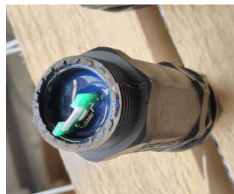
Fig. 2 Sensor for measuring the relative humidity at different depth of the wood-based material by the sorptive method
