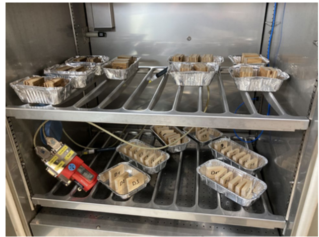
Fig. 7 Test specimen in the climate chamber with data logger to check the actual boundary conditions (temperature and humidity)
