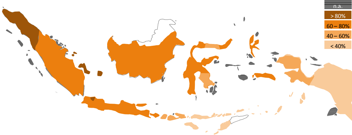
Figure 2 Indonesian electrification ratios (number of electrified households) per province. Own graph based on data from 2011 from the Indonesian Ministry of Energy and Mineral Resources (Kusdiana 2012; Winoto et al. 2012)
