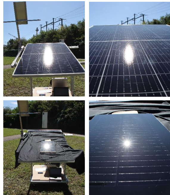
Figure 10: Phenomenological approach to show the independence of horizontal and vertical axis of the glare ellipse from the distance of the observer for standard (upper row) and float module (lower row)
