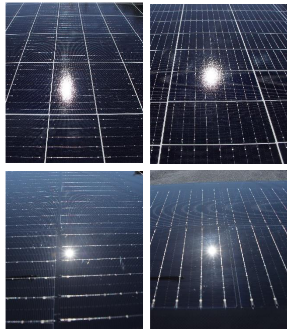
Figure 11: Phenomenological approach to investigate the influence of PV module orientation on the horizontal and vertical axes of the glare ellipse for standard (top row) and float (bottom row) modules.
