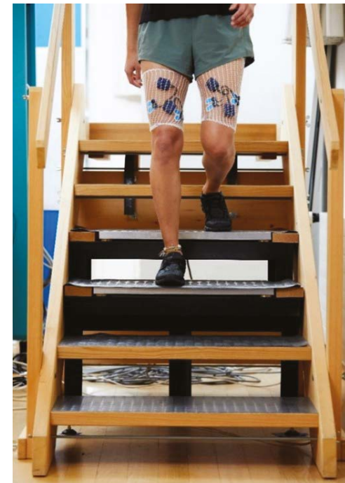
Figure 14: Stair descent on instrumented stairway with force plates embedded to third and fourth step (symbolic image as another device for EMG measurements was used in PhD project) (©Bern Movement Lab)
