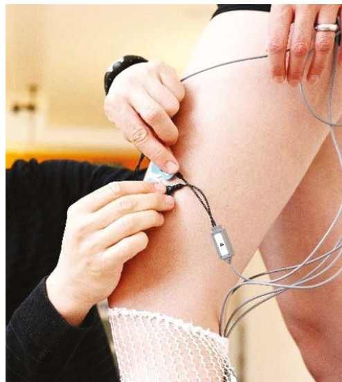
Figure 13: Connecting cables with electrodes and fixation of cables and preamplifier with elastic, mesh-like tubular bandage (©Bern Movement Lab)
