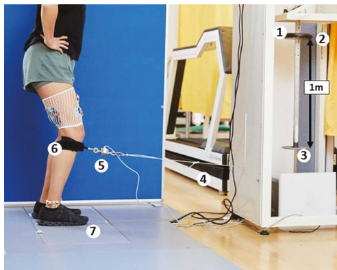
Figure 3: Stretch reflex measurements in upright standing position (©BFH Bern Movement Lab) Legend (Fig. 3): 1) electromagnet, 2) falling barbell weight, 3) stopper, 4) wire rope, 5) force transducer, 6) brace, 7) two force plates
