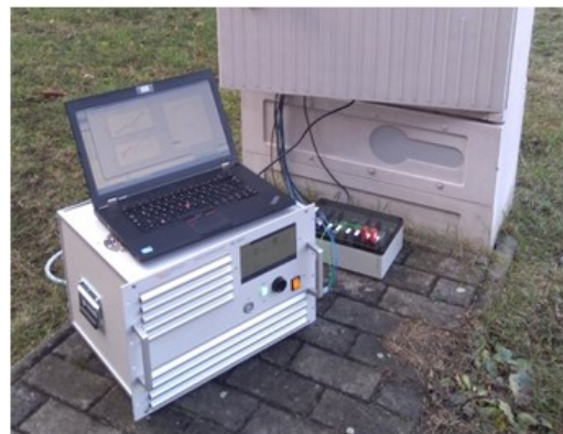
Fig. 4: Measurement system while measuring at a junction box.
