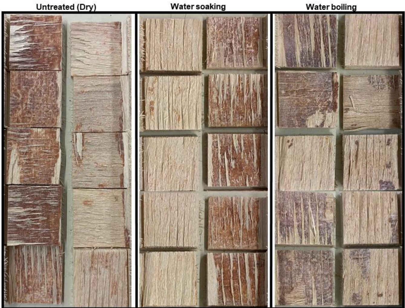
Figure 5. Fractured surface of the plywood bonded with MOC binder after shear strength test.
