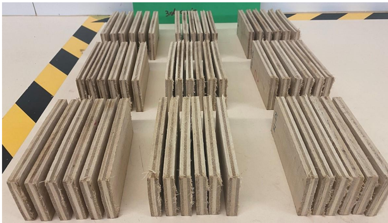
Figure 8. Plywood samples after third cycle of delamination testing according to ANSI/HPVA HP-1, 2020.
