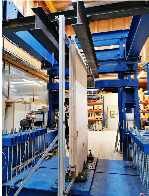
Fig. 26 Lateral stabilisation by plastic rollers
