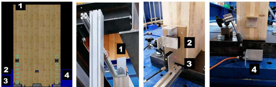
Fig. 24 Position of the lasers—1: Horizontal at the top of the wall—2 and 3: Vertical and horizontal laser at the bottom of the wall—4: Vertical at the bottom of the wall
