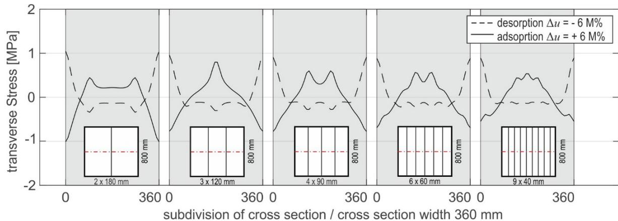
Figure 10: Transverse stresses due to moisture step loading in cross-laminated beams with identical cross-sections but different set-up regarding number of single beams.
