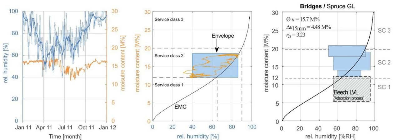
Figure 2: Evaluation of envelope of ambient climate and moisture content for timber bridges, left: moisture content and relative humidity on a specific timber bridge, middle: analyses of data compared with equilibrium moisture content (EMC), right: summary of four analysed timber bridges monitored by BFH
