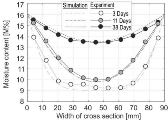
Figure 4: Numerical distribution of moisture content in comparison to experimental results on a glued laminated cross section of 90 x 270 x 16 mm<sup>3</sup> under adsorption process from 9 to 16 M% done by Jönsson [13]
