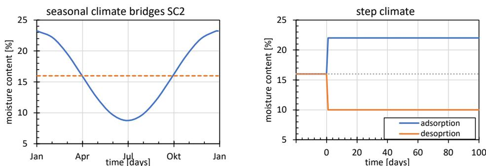
Figure 3: Simplified seasonal climate for bridges (left), stepwise climate change used for numerical simulation (right)
