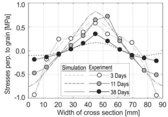
Figure 5: Numerical stress distribution and development in comparison to experimental results on a glued laminated cross section of 90 x 270 x 16 mm<sup>3</sup> under adsorption process from 9 to 16 M% done by Jönsson [13]
