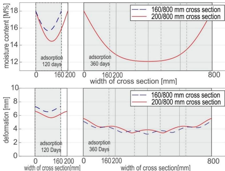
Figure 8: Moisture content distributions (top) and deformation across the width of the timber beams of different widths subjected to a step load of 6 M% moisture content increase. All beams have a height of 800 mm and the duration of the simulations is indicated in the figures.
