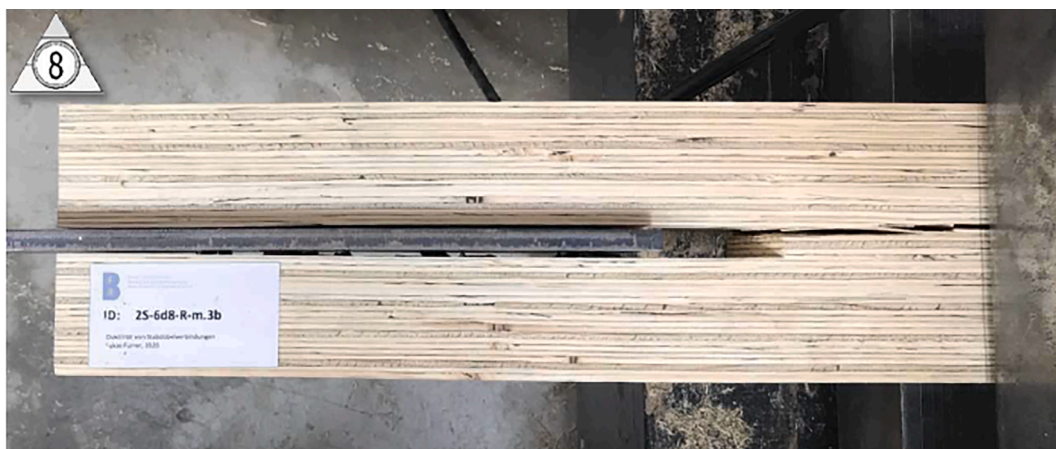
Fig. 8. Specimen split along the slot line (bracket - type opening) after the monotonic test.
