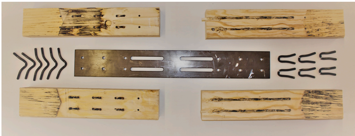
Fig. 25. Individual parts of the specimen with S235JR after the monotonic test.
