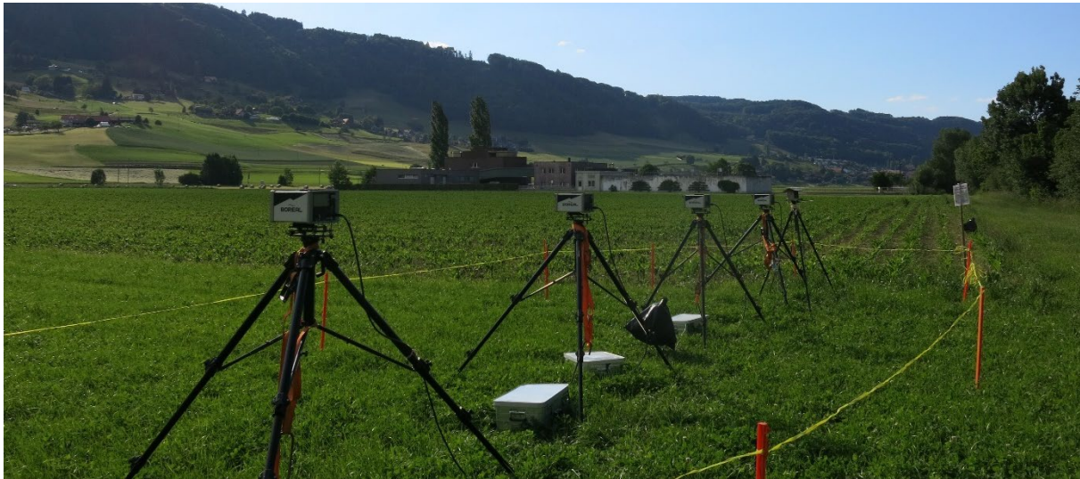
Figure 3 Fixation of GasFinder with clamping set during the intercomparison measurements at WWTP-2.
