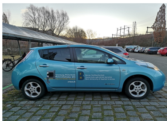
Figure 1: Research e-vehicle Nissan Leaf of the PV LAB at BFH (Burgdorf-Switzerland) showing photovoltaic reference cell measures irradiance levels on the right side of the car. Source: PV LAB at BFH.
